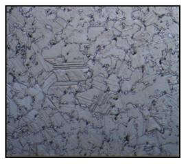
**Figure 6.** Microstructure of cobalt based superalloy (100x – electrolytic etched with 6% chromic acid + 10% HCl)
