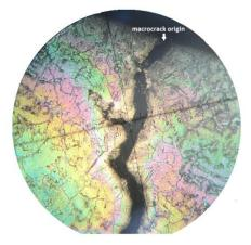
**Figure 5.** Microstructure of macro crack zone (100x - e) electrolytic etched with 6% chromic acid + 10% HCl)
