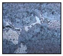
**Figure 14.** Microstructure of microcrack tip (200x - electrolytic etched with 6% chromic acid + 10% HCl)
